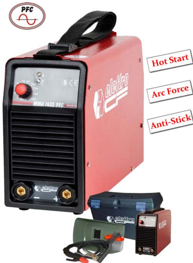
This INVERTER portable power source has been designed for maintenance operations and assembling of external plants. It can be also connected to household mains or to generators with an electronic regulator of the tension (not greater than 260V RMS) and a power equal to or greater than 5 kVA.
