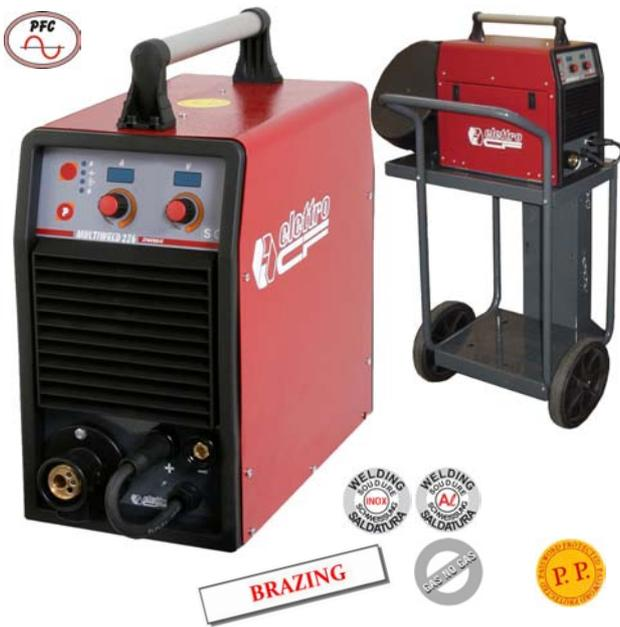
**MULTIWELD 236 SYNERGIC** is a **single-phase multipurpose inverter** power source, suitable for **welding alternately in MIG/MAG, MMA (stick electrode) and DC TIG ("lift" start) mode**. It has a **compact design**, a **low weight** and, with a **welding current of 220A**, allows to weld wires up to a diameter of 1,2mm. It can be **connected to generators**.
