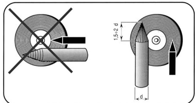
Grind the electrode tip so that it has vertical grooves as shown in the figure.
