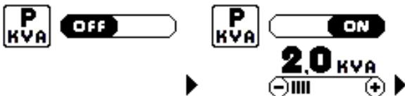
The factory default mode is OFF meaning that there is no limitation to the absorbed input power.
