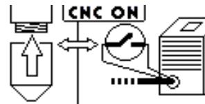
If this picture appears the machine is reporting that the START CNC function is active and it is necessary to check whether the nozzle holder has been removed and/or that the automatic torch's external contact has stayed open (in fact it needs to be short circuited for correct start-up from cnc)
