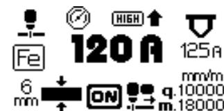
It is nevertheless possible to set the function on OFF, so as to read and adjust the torch's work pressure to the required value (within the pre-set limits) directly from the main panel which will appear as follows:
