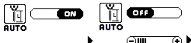
The factory default mode is AUTO ON which allows the power source to automatically and synergically adjust the length of the pilot arc based on the mounted torch, the installed consumables and the selected processing procedure. It is nevertheless possible to set this function on OFF so as to be able to manually adjust pilot arc length.
