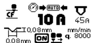
The power source automatically displays the width and depth of the groove that can be achieved with the current values (Pict. 4 Ref. G) at the relative processing speed (Pict. 4 Ref. E) set by the operator, and tells you which nozzle to use (Pict. 4 Ref. F).
