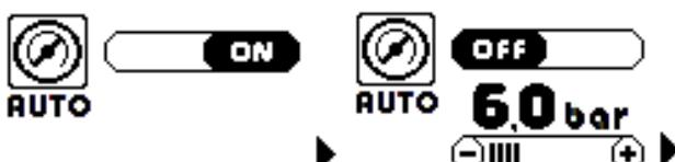
The factory default mode is AUTO ON which allows the power source to maintain the torch's work pressure at the best value, also in the presence of variations of the inlet pressure.
